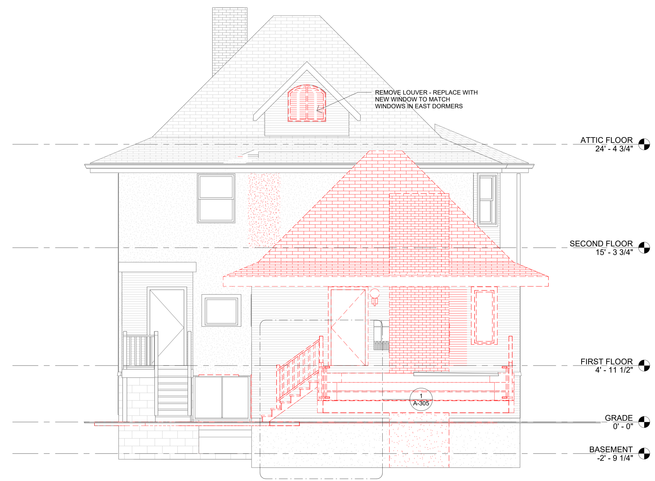
1 WEST ELEVATION SELECTIVE DEMOLITION 1/4" = 1'-0"
