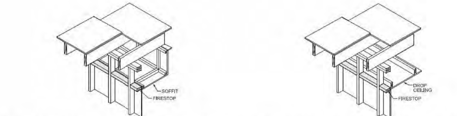
Figure R302.11(3) FIRESTOPPING—FURRED SOFFIT
